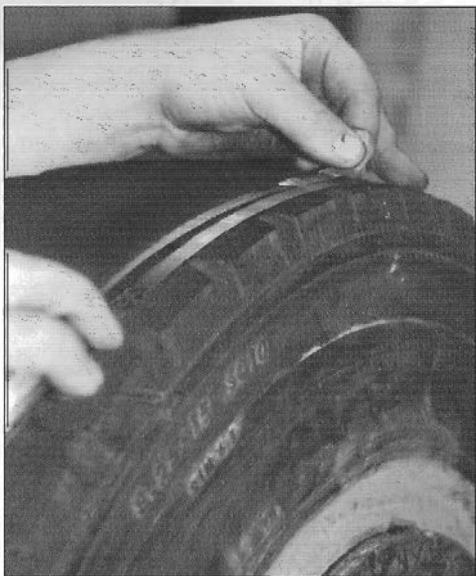
Photo II - The buffed diameter is checked closely on both shoulders. Tires worn too far are built up or rejected.
