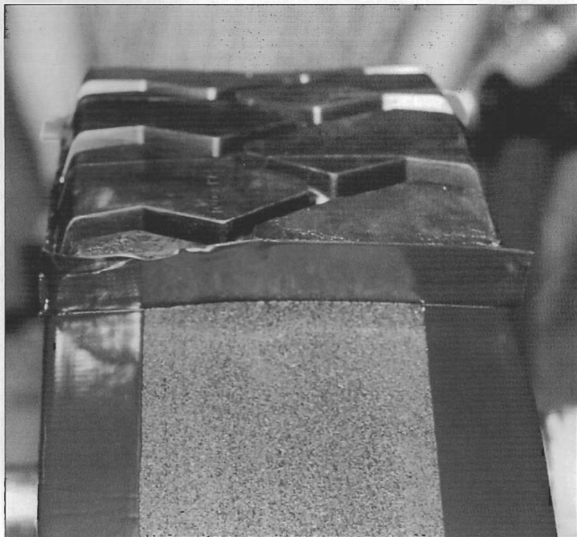
Photo V - After application to the casing, the tread is thoroughly stitched down.
