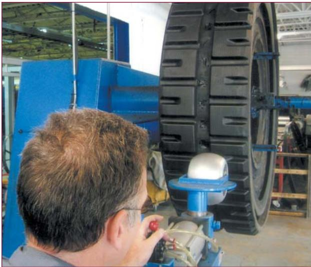
After the bonding gum and the two pre-cured treads have been applied, it is thoroughly stitched.
