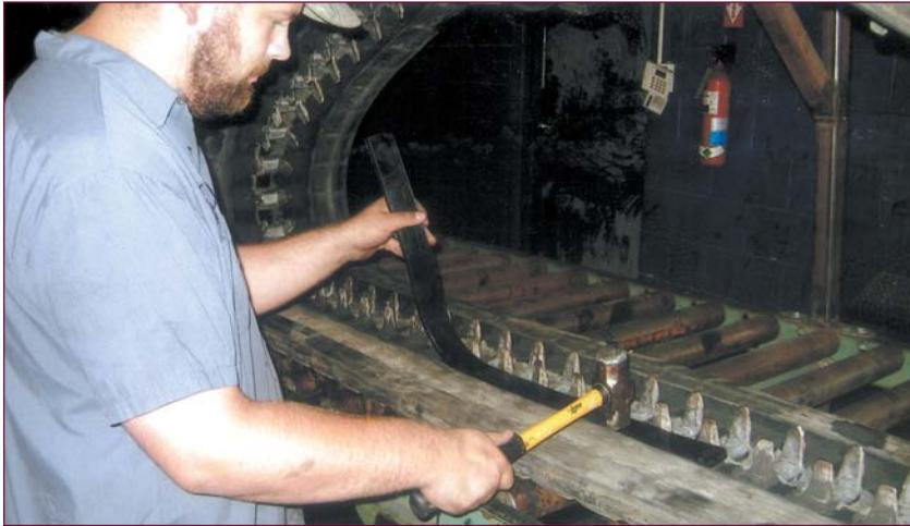
**Above:** Repair technician Don Fry applies replacement rubber to bond to the steel and rubber in the track
