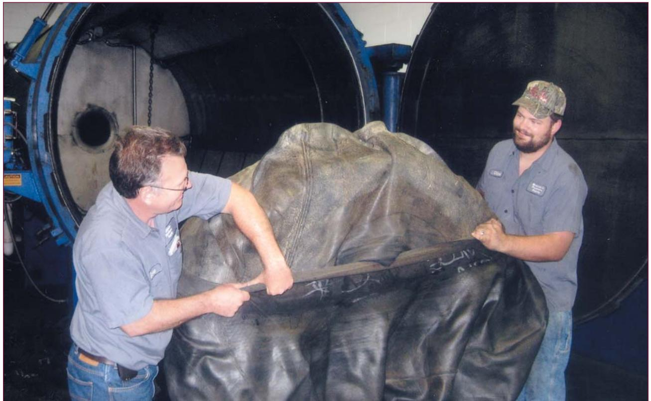
An envelope is applied before the track is cured in the autoclave shown in the background.
